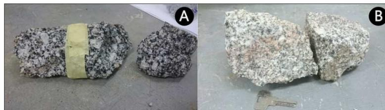
**Figure 3 (A): Hand Specimen (Mu-28) Shows the Heterogeneity and General Appearance of an Unweathered Muhtadi Rock With Feldspar Megacrysts. Tape Width is 2 Cm. (B) Hand Specimen (Wa-5) Shows the Homogeneity and the General Appearance of an Unweathered Wa'ara Rock. No Feldspar Megacrysts and Less Mafic Assembly.**
